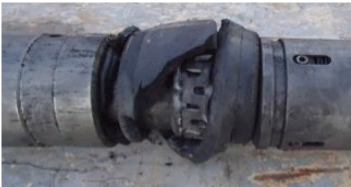
Retrievable solid elastomer bridge plugs that have experienced downhole failure a) compression set, b) Rapid Gas Decompression
