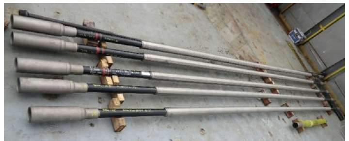
Five joints of 20-ft sand screen were installed in the deviated well within three days without any HSE or operational issues.
