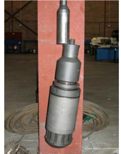
▲ Workshop demonstration: A 2.220" HTHS Magnet used to pick up a 7" GS Pulling Tool. Clean end-to-end contact not necessary.
